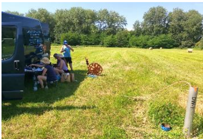
Fig.12. Cleansing pumping of a piezometer DW-7.
